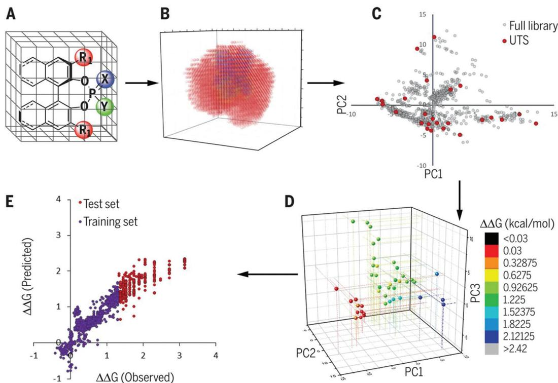
**Fig. 11** Chemoinformatics-guided optimization protocol. (A) Generation of a large *in silico* library of catalyst candidates. (B) Calculation of robust chemical descriptors. (C) Selection of a universal training set (UTS). (D) Acquisition of experimental selectivity data. (E) Application of ML to use moderate- to low-selectivity reactions to predict high-selectivity reactions. Reproduced with permission from ref. 17. Copyright 2019 American Association for the Advancement of Science.
