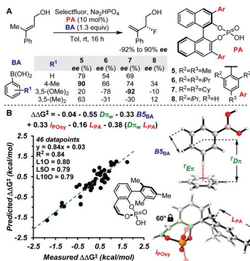
**Fig. 15** Parametrization of non-covalent interactions in enantioselective fluorination of allylic alcohols reported by Toste and Sigman *et al.* (A) Reaction scheme and substituent effects of boronic acids and chiral phosphate anions on the enantioselectivity. (B) Multivariate model correlating the stereoselectivities from catalysts 5–8 and 18 different boronic acids. Adapted with permission from *J. Am. Chem. Soc.*, 2017, **139**, 6803. Copyright 2017 American Chemical Society.
