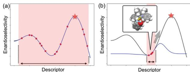
**Fig. 10** Schematic representation of (a) Type II vs. (b) Type I QSPR in molecular design. Black and blue lines are true functions and regression models, respectively. Red points and red stars are training samples and target molecule, respectively. The pale red region is the applicability domain of regression models.
