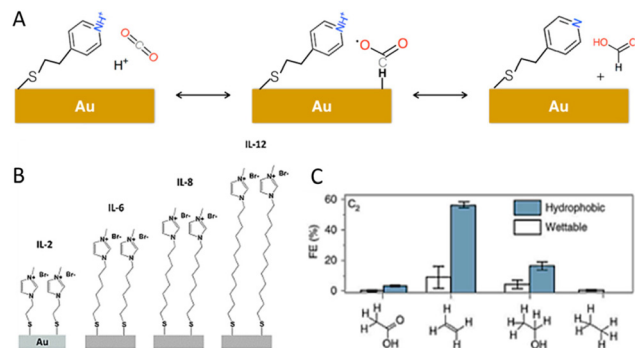
Fig. 20 Comparison of partial current density and FE for thiolate ligands on polycrystalline Au: (A) proposed reaction mechanism of the formate production at 4-PEM and Au interfaces. (B) Schematic of Au electrodes with 1-methylimidazolium-terminated SAMs (IL-2, IL-6, IL-8, and IL-12). (C) FE of C 2 products on both wettable and hydrophobic Cu dendrites at the total current density of 30 mA cm -2 . Adapted from ref. 175, 171 and 168 with permission. Copyright 2017 American Chemical Society, 2015 Royal Society of Chemistry and 2019 Nature Publishing Group.
