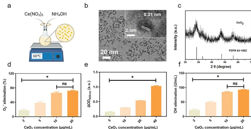
**Fig. 1** The characterization analysis and enzyme-mimicking activities of CeO<sub>2</sub> NPs. (a) Synthesis scheme of CeO<sub>2</sub>; (b) TEM images; (c) XRD spectrum; (d) SOD-like activity of CeO<sub>2</sub> NPs at different concentrations; (e) CAT-like activity; and (f) <sup>•</sup>OH elimination ability. ns means  $P > 0.05$  and \* means  $P < 0.05$ .
