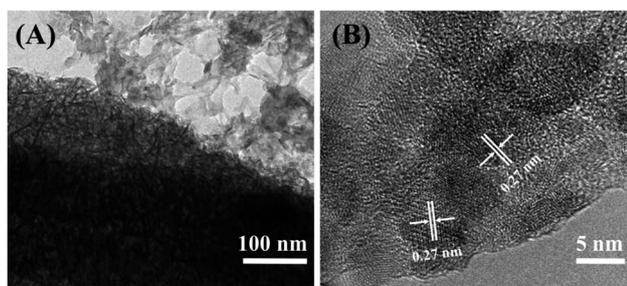
Fig. 3 (A) TEM image of the Ppy/MnO<sub>2</sub> nanocomposite; (B) high-resolution TEM image of the Ppy/MnO<sub>2</sub> nanocomposite. Reproduced from ref. 50 with permission from Elsevier, Copyright © 2016.
