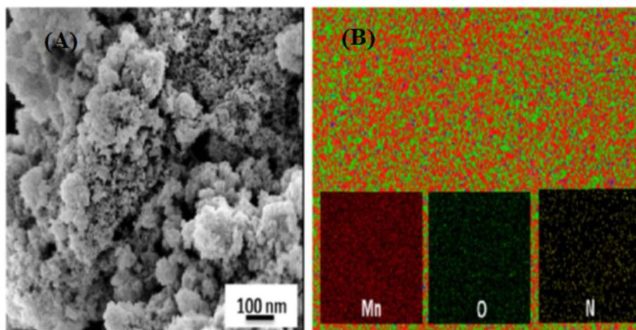
Fig. 5 (A) FESEM image and (B) elemental map of the MnO<sub>2</sub>/Ppy nanocomposite. Reproduced from ref. 56 with permission from Elsevier, Copyright © 2015.
