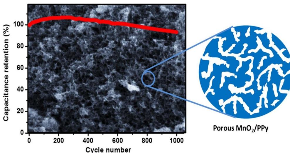
Fig. 7 Cycling stability of the fabricated symmetric MnO<sub>2</sub>/Ppy supercapacitor device. Reproduced from ref. 56 with permission from Elsevier, Copyright © 2015.
