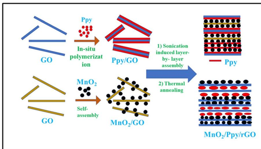
Fig. 4 Schematic diagram of formation of (MnO<sub>2</sub>, Ppy)/rGO composites.
