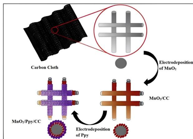
Fig. 2 Schematic view of the fabrication process of the flexible Ppy/MnO<sub>2</sub> composite electrode. Reproduced from ref. 50 with permission from Elsevier, Copyright © 2016.
