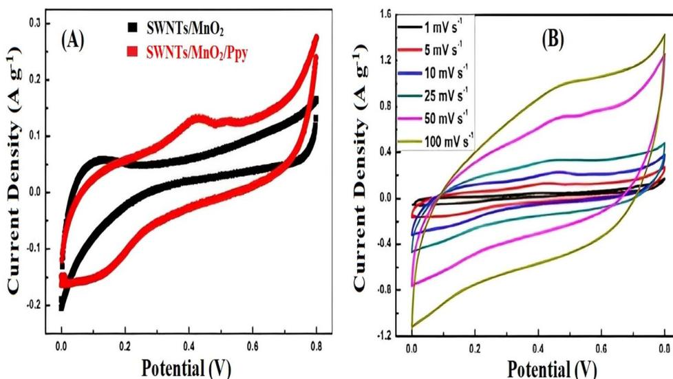
Fig. 6 (A) Comparison of the CV curves of single-walled nanotubes (SWNTs)/MnO<sub>2</sub> and SWNTs/MnO<sub>2</sub>/Ppy at a scan rate of 5 mV s<sup>-1</sup> (B) SWNTs/MnO<sub>2</sub>/Ppy electrode CV curves at various scan rates. Reproduced from ref. 58 with permission from Elsevier, Copyright © 2014.
