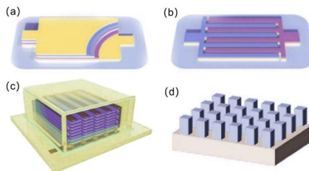
**Fig. 2** Schematic diagrams of various micro-LIBs according to different cell microstructures: (a) laminated thin film structure, (b) planar interdigital structure, (c) 3D interdigital structure, (d) other types of 3D architecture (microtube structure).
