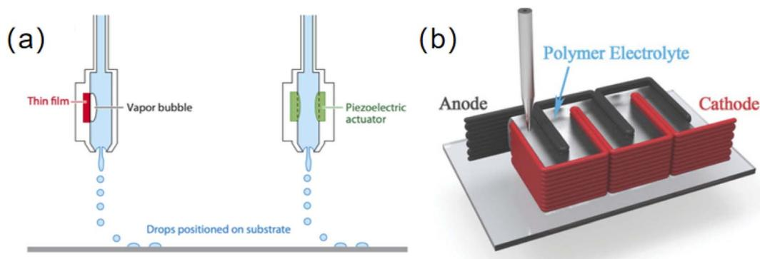
Fig. 8 (a) Schematic diagram of inkjet printing. (b) Schematic of a DIW-printed 3D micro-LIB. Reproduced with permission from ref. 70, Copyright© 2016, WILEY-VCH Verlag GmbH & Co.
