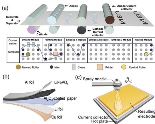
Fig. 6 (a) Schematic diagram of flexographic printing and (b) a thin-film lithium metal battery based on the flexographic printed  $\text{LiFePO}_4$  cathode. Reproduced with permission from ref. 62, Copyright© 2022, Wiley-Blackwell. (c) Schematic diagram of spray printing for preparing thin film electrodes of LIBs. Reproduced with permission from ref. 63, Copyright© 2018, Elsevier Ltd.
