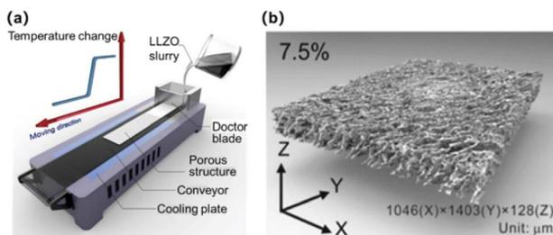
Fig. 5 (a) Schematic diagram of the tape-casting technique. (b) Porous  $\text{Li}_7\text{La}_3\text{Zr}_2\text{O}_{12}$  solid electrolyte prepared by tape-casting. Reproduced with permission from ref. 60, Copyright© 2020, American Chemical Society.
