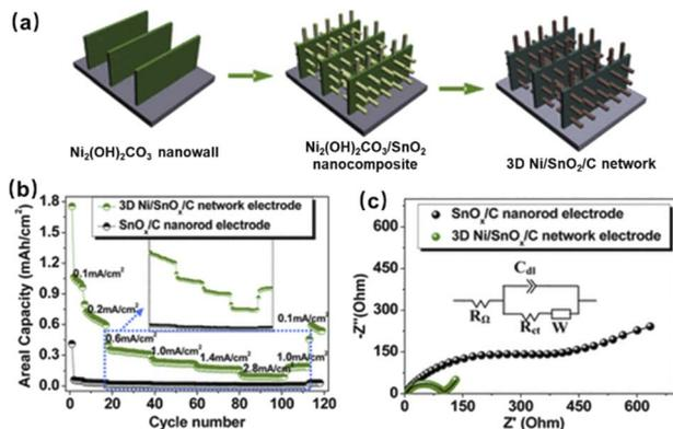
Fig. 11 (a) Fabrication process, (b) rate performance and (c) EIS plot of the 3D Ni/SnO<sub>x</sub>/C electrode. Reproduced with permission from ref. 81, Copyright© 2013, American Chemical Society.
