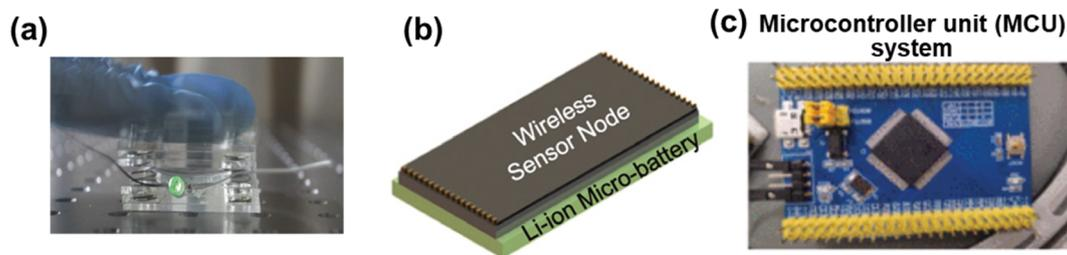
Fig. 17 (a) Photograph of a green light-emitting diode lit by a self-powered microsystem. Reproduced with permission from ref. 137, Copyright© 2017, Wiley-VCH Verlag. (b) Schematic diagram of a wireless sensor and a micro-LiB integrated device. Reproduced with permission from ref. 139, Copyright© 2021, Elsevier B.V. (c) Photograph of a smart light-working microcontroller unit.
