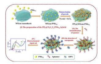
Fig. 4  $PPy@Ti_3C_2Tx/PMo_{12}$  sensor fabrication and working process diagram. Copied with permission.9 Copyright 2019, with permission from Elsevier.
