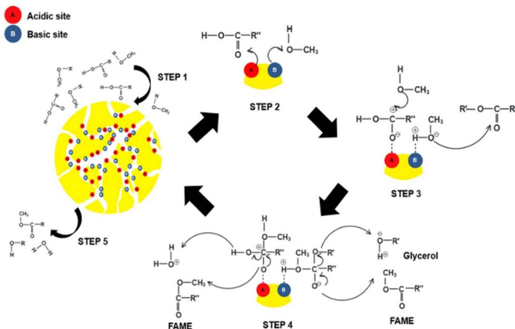
Fig. 6 The reaction mechanism of biodiesel production using a bifunctional acid–base catalyst.<sup>83</sup>
