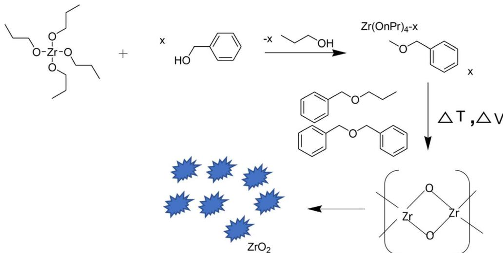
Fig. 3 Reaction mechanism of the nonaqueous synthesis of ZrO<sub>2</sub> nanoparticles.<sup>28</sup>
