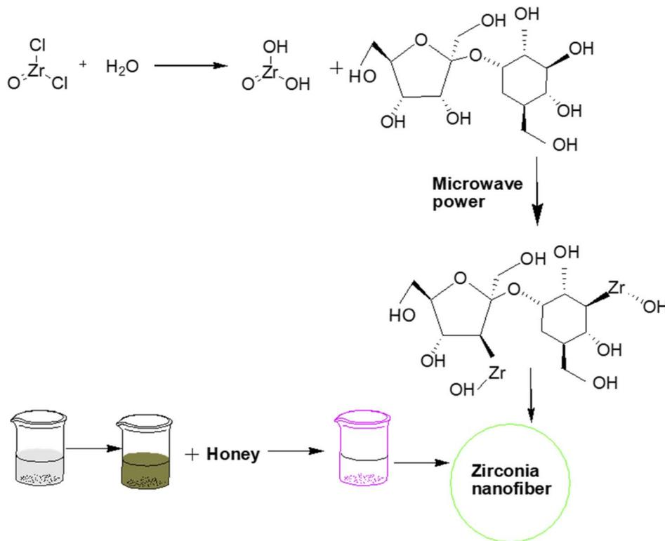
Fig. 1 Honey mediated microwave assisted sol–gel synthesis of stabilized zirconia nanofibers.<sup>18</sup>
