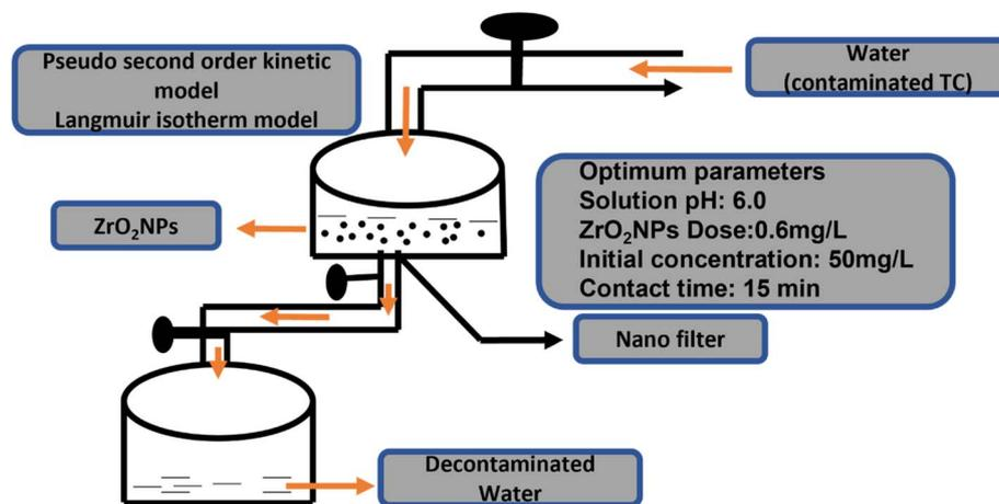
Fig. 11 Schematic diagram of batch adsorption of TC on the surface of biosynthesized ZrO<sub>2</sub> NPs.<sup>66</sup>
