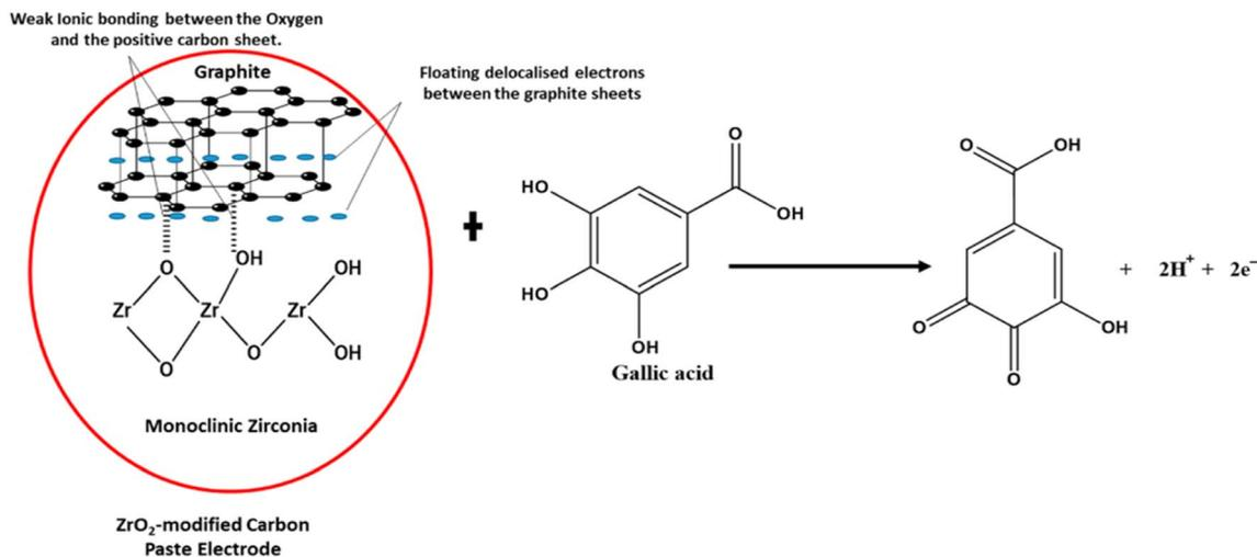
Fig. 14 Proposed interaction between ZrO<sub>2</sub> NPs and graphite, demonstrating a weak ionic bond between some of the oxygen and the positive graphite sheet in the electrochemical determination of gallic acid.<sup>133</sup>
