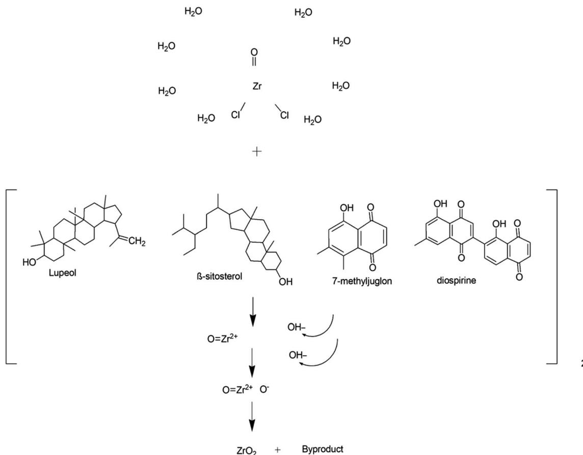
Fig. 5 Proposed reaction mechanism of synthesis of zirconia nanoparticles.<sup>57</sup>
