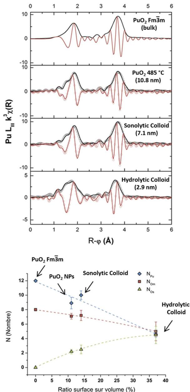
Fig. 15 Top: FT magnitudes of experimental  $k^3$ -weighted EXAFS spectra acquired at the Pu L<sub>3</sub> edge on PuO<sub>2</sub> nanoparticles in comparison to a reference (black curve, data obtained in the 2–14 Å<sup>-1</sup> range). Bottom: correlation of the coordination numbers obtained for the three Pu–O distances used to fit the Pu–O shell as a function of the S/V ratio of the nanoparticle. Adapted from ref. 96 with permission from Nature Publishing Group, copyright 2017.
