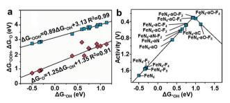
Fig. 5 (a) The scaling relations of  $\Delta G_{^*\rm OOH}$  vs.  $\Delta G_{^*\rm OH}$  and  $\Delta G_{^*\rm O}$  vs.  $\Delta G_{^*\rm OH}$ . (b) A volcano plot for the ORR overpotential against the adsorption energy  $\Delta G_{\star_{OH}}$ , wherein the letter "a" denotes the axial ligands and the subscripted number denotes the number of fluorine atoms that are embedded into graphene layers.
