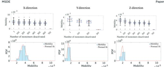
Fig. 5 Effect of removal of highly ranked monomers on mobility distribution. The first row shows the decrease in mobility with the removal of each monomer. The second row represents the mobility distribution just before the last connecting monomer is removed.
