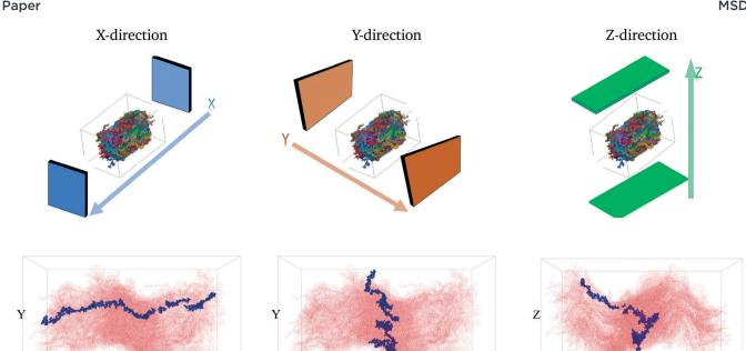
Fig. 3 The first row shows the respective source and drain electrodes in each direction. The second row shows the corresponding representative pathways in each direction.
