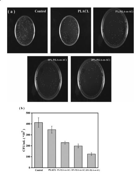
Fig. 9 Assessment of the bacteriostasis properties: (a) photographs of E. coli colonies; (b) colony counts.
