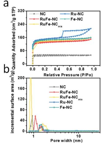
Fig. 1 (a) Nitrogen sorption isotherms of RuFe-NC, RuFe-NC<sub>mix</sub>, Ru-NC, Fe-NC, and NC, and (b) the corresponding pore size distribution profiles.
