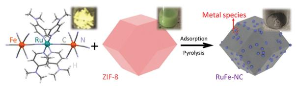
Scheme 1 Molecular structure of the Ru(LFe)<sub>2</sub> complex and the synthetic procedure of the RuFe-NC composite. Insets show the photographs of the products at different reaction stages.
