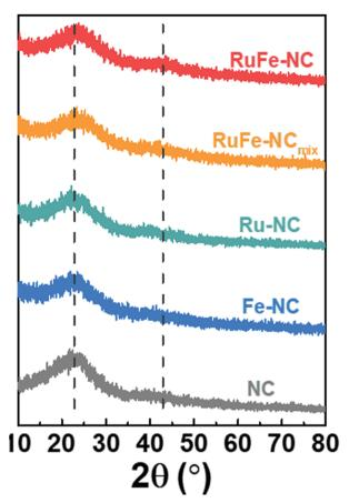
**Fig. 3** XRD patterns of RuFe-NC, RuFe-NC<sub>mix</sub>, Ru-NC, Fe-NC, and NC. The dashed lines indicate the expected  $2\theta$  position of the (002) and (100) diffractions of graphite (JCPDS No. 01-0646). Units on the *y*-axis have arbitrary units.
