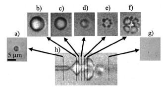
Fig. 2 Optical frame (a–g) and streak (h) images showing the oscillation and fragmentation of an ultrasound contrast agent microbubble. The microbubble has an initial diameter of 3  $\mu$ m (a), and the streak image (h) shows the changes in the bubble diameter as a function of time and the ultrasound pressure wave, with the fragmentation occurring during compression (e and f). Reprinted with permission from ref. 53.
