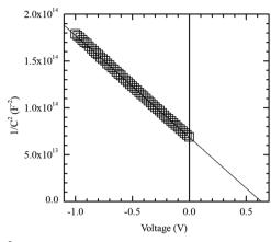
Fig. 5  $\,$   $C^{-2}$  vs. voltage plot (Mott–Schottky plot) of the 2  $\times$  2 cm² solar cell. From the x-axis crossing point, a  $V_{\rm bi}$  of 683 mV is deduced indicating an inverted surface.
