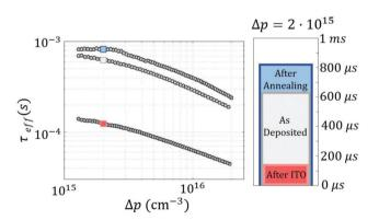
Fig. 2 Effective carrier lifetime ( $\tau_{\text{eff}}$ ) as a function of the excess carrier density  $(\Delta p)$  of c-Si(n) substrate, with asymmetrically passivated front and back surfaces using ALD  $V_2O_5$  and ALD  $Al_2O_3$  films, respectively. Bar plot shows the  $\tau_{\rm eff}$  values at  $\Delta p = 2 \times 10^{15} \ {\rm cm}^{-3}$
