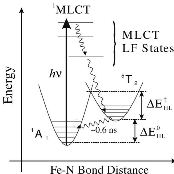
Fig. 2 Configuration-coordinate diagram for photoexcited  $\text{Fe}(\text{bpy})_3$ , one example of a spin-crossover molecule. The transition to a high-spin electronic state of the Fe ion occurs via a higher energy MLCT state that is directly excited by the absorption of a visible or UV photon. Reprinted with permission from ref. 40 [Gawelda *et al.*, *Phys. Rev. Lett.*, 2007, **98**, 054401]. Copyright 2007 by the American Physical Society.
