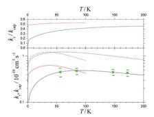
Fig. 7 Reaction probabilities  $k_{\rm r}/k_{\rm cap}$  (upper panel), capture rate constants  $k_{\rm cap}$  (lower panel, dashed curves) and reaction rate constants  $k_{\rm r}$  (lower panel, solid curves), from  $f_{\rm el}(T)$ -corrected BO (blue curves) and NBO (red curves) calculations of the present work, in comparison to experimental results from ref. 33 (green symbols with error bars).
