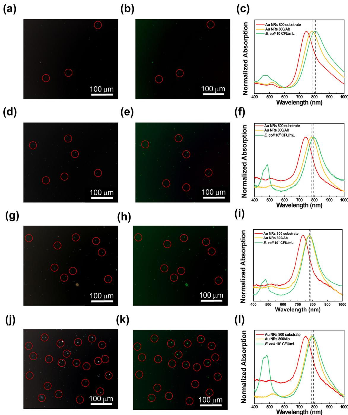
Fig. 6 Characterization of the bioactive plasmonic substrates after incubating *E. coli* dispersions in minimum E at different cell concentrations. Contrast phase microscopy images (a, d, g and j), fluorescence microscopy images (b, e, h and k), and absorption spectroscopy characterization (c, f, i and l) of the bioactive plasmonic substrate progressively incubated in a  $10$ ,  $10^2$ ,  $10^3$ , and  $10^4$  CFU mL<sup>-1</sup> *E. coli* cell dispersion.
