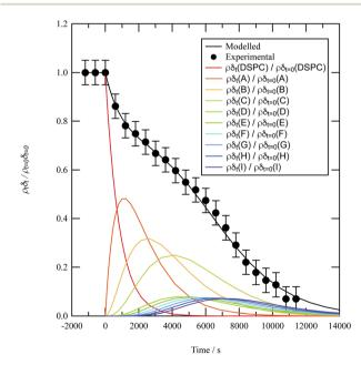
Fig. 8 Experimental (black circles) and modelled (black line) reaction profiles for the lipid DSPC being oxidised by OH radical at the airwater interface. The coloured lines represent the individual reaction profiles for the species DSPC, A, B, C, ..., H, I, J at the air-water interface for reaction 10. The sum of these coloured profiles is equal to the modelled reaction profile represented by the black line.
