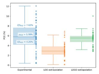
Fig. 5 PCE distribution of non-fullerene acceptors in our database, indicating the lower quartile (Q1<sub>PCE</sub>), median ( $\mu_{PCE}$ ) and upper quartile (Q3<sub>PCE</sub>). We also show the predicted PCE distributions with LOOextrapolation and LOGO-extrapolation.
