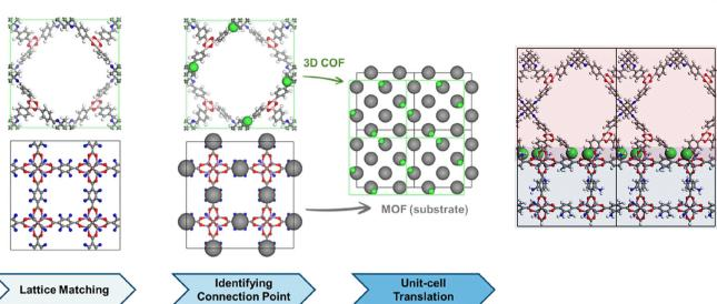
Fig. 4 Three steps for heteroepitaxial growth of 3D COFs on MOFs and the final structure. Reprinted with permission from ref. 40. Copyright (2021) American Chemical Society.
