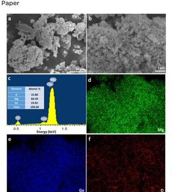
Fig. 4 SEM characterisation of Mg<sub>2</sub>Ge powders synthesised from Mg and Ge at 200 W with an irradiation time of 60 s, showing: (a and b) SEM images at different magnification: (c) a representative EDX spectrum taken from the area shown in the image in (b): and (d-f) elemental maps of Mg, Ge and O, respectively, taken from the same area shown in (b).
