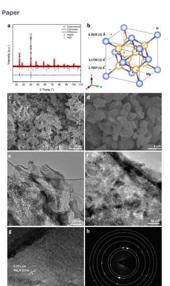
Fig. 1 Results from PXRD and electron microscopy for the MIMP-synthesised  $Mg_2Si$  powders, showing (a and b) profile plot of the Rietveld refinement against PXD data and the corresponding crystal structure; (c and d) SEM images, (e–g) TEM images, and (h) SAED pattern taken from the area shown by the image in (g).
