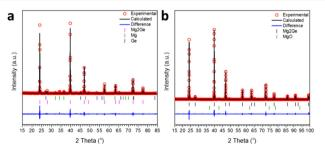
Fig. 3 Profile plot of the Rietveld refinements against PXRD data for Mg<sub>2</sub>Ge samples synthesised at 200 W with a MW irradiation time of: (a) 30 s and (b) 60 s, respectively.
