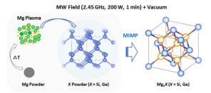
Scheme 1 Schematic of the principal Mg plasma-enabled reaction route proposed for the MIMP synthesis of Mg<sub>2</sub>Si and Mg<sub>2</sub>Ge.
