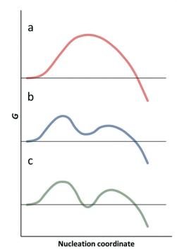
Fig. 4 Gibbs energy profiles for classical nucleation (a), and two-step nucleation with metastable clusters (b) and stable clusters (c).
