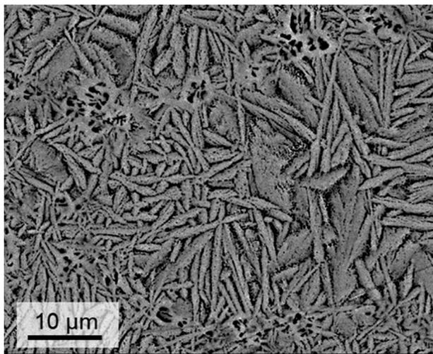
Fig. 19 Microstructure of a sinter crystallized sample with the composition 8 BaO·8 SrO·35 ZnO·45 SiO<sub>2</sub>·1 ZrO<sub>2</sub>·1 La<sub>2</sub>O<sub>3</sub>·2 B<sub>2</sub>O<sub>3</sub> sintered at 800 °C for 1 h. Redrawn from ref. 45.
