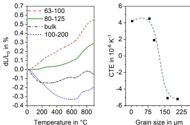
Fig. 20 Thermal expansion of sinter crystallized glass powders with the composition 8 BaO·8 SrO·35 ZnO·45 SiO<sub>2</sub>·1 ZrO<sub>2</sub>·1 La<sub>2</sub>O<sub>3</sub>·2 B<sub>2</sub>O<sub>3</sub> sintered at 950 °C for 1 h. Left: Dilatometric measurements. Right: CTE vs. grain size of sintered powders. The dashed line is just a guide for the eyes. Redrawn from ref. 45.
