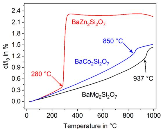
Fig. 4 Comparison of the dilatometric thermal expansion of  $\text{BaZn}_2\text{Si}_2\text{O}_7$ ,  $\text{BaCo}_2\text{Si}_2\text{O}_7$ , and  $\text{BaMg}_2\text{Si}_2\text{O}_7$ .
