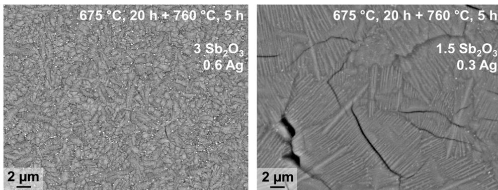
Fig. 16 SEM micrographs of glasses from the system BaO-SrO-ZnO-SiO<sub>2</sub> nucleated with Ag + Sb<sub>2</sub>O<sub>3</sub> in different concentrations after a two-step thermal treatment. Both micrographs show the same magnification.
