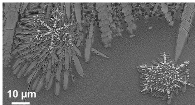
Fig. 18 SEM micrograph with the composition 9.4 BaO-9.4 SrO-37.6 ZnO-37.6 SiO<sub>2</sub>-4 P<sub>2</sub>O<sub>5</sub>-2 Ce<sub>2</sub>O<sub>3</sub>, crystallized at 690 °C for 20 h and subsequently at 850 °C for 1 h.
