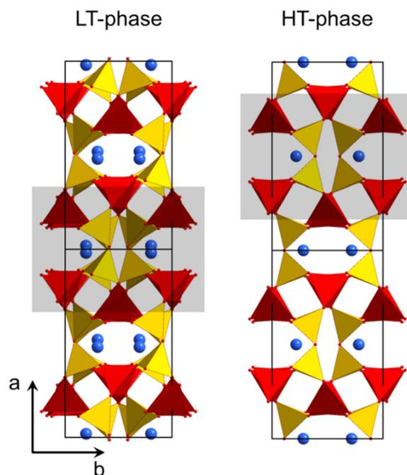
Fig. 2 Crystal structure of LT- and HT-BaZn<sub>2</sub>Si<sub>2</sub>O<sub>7</sub>.<sup>1,21</sup> The grey rectangles mark similar structural units, which convert into each other during phase transition.
