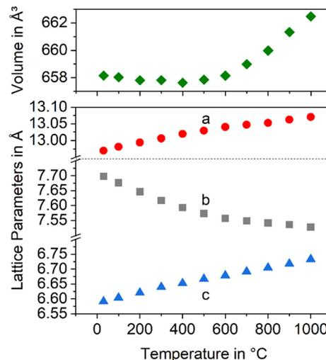
Fig. 8 Lattice constants and unit cell volume of the Ba<sub>0.6</sub>Sr<sub>0.4</sub>Zn<sub>2</sub>Si<sub>2</sub>O<sub>7</sub> solid solutions as a function of temperature.
