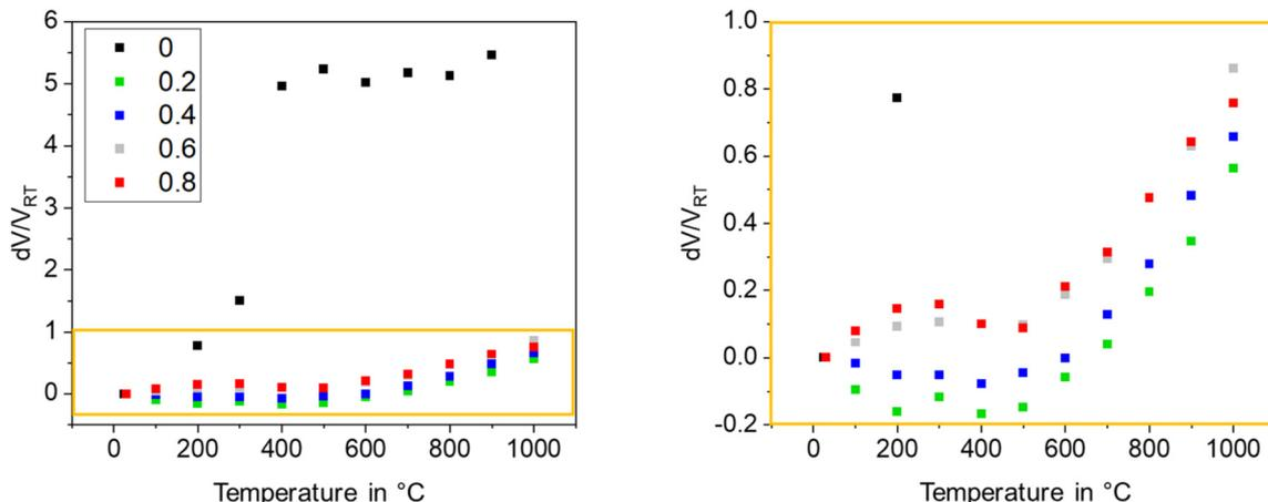
Fig. 7 Thermal expansion of Ba<sub>1-x</sub>Sr<sub>x</sub>Zn<sub>2</sub>Si<sub>2</sub>O<sub>7</sub> as a function of the temperature for various *x*-values.
