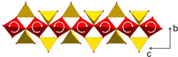
**Fig. 9** Part of the network formed by  $\text{ZnO}_4$  (red) and  $\text{SiO}_4$  tetrahedra (yellow). With increasing temperature,  $\text{ZnO}_4$  tetrahedra rotate, which results in a stretching of the  $\text{ZnO}_4$ -chain in the direction of the  $c$ -axis and a shortening in the  $b$ -direction. Redrawn from ref. 9.
