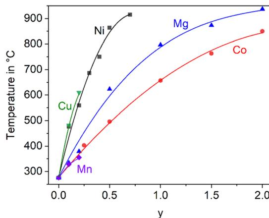
Fig. 5 Temperature of the phase transition for solid solutions of  $\text{BaZn}_{2-y}\text{M}_y\text{Si}_2\text{O}_7$  with  $\text{M} = \text{Co}, \text{Cu}, \text{Mg}, \text{Mn},$  and  $\text{Ni}$ .<sup>2,5,22,23</sup> The lines are drawn as a guide for the eyes.
