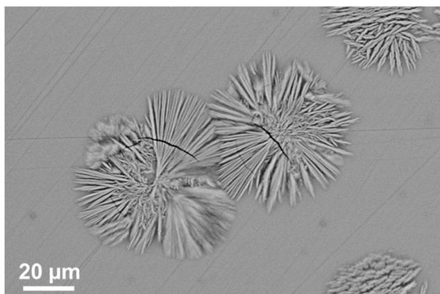
Fig. 17 Microstructure of a sample with the composition 7.5 BaO-7.5 SrO-34 ZnO-43 SiO<sub>2</sub>-7 ZrO<sub>2</sub>-1 TiO<sub>2</sub> crystallized at 750 °C for 48 h and at 840 °C for 30 min.
