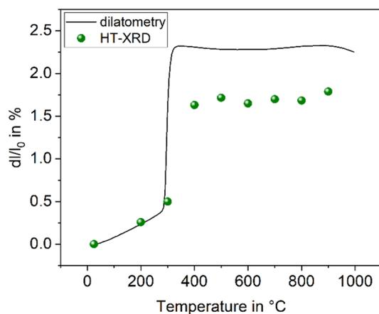
Fig. 1 Thermal expansion of BaZn<sub>2</sub>Si<sub>2</sub>O<sub>7</sub>. Redrawn based on ref. 5.
