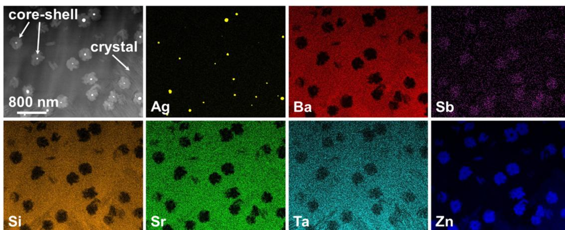
Fig. 15 STEM micrograph and elemental distribution of core-shell structures within a glass with the molar composition 9.5 BaO·9.5 SrO·38 ZnO·38 SiO<sub>2</sub>·3.2 Ta<sub>2</sub>O<sub>5</sub>·1.5 Sb<sub>2</sub>O<sub>3</sub>·0.3 Ag after a two-step heat treatment at 675 °C for 10 h and 760 °C for 5 h and related EDX maps. The main crystal phase (denoted as “crystal”) is composed of Ba<sub>0.5</sub>Sr<sub>0.5</sub>Zn<sub>2</sub>Si<sub>2</sub>O<sub>7</sub>.
