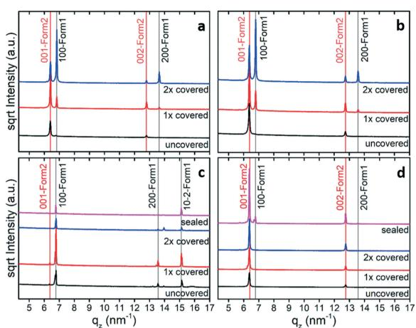
Fig. 1 Specular X-ray diffraction pattern for phenoxazine crystallized on a silicon oxide surface. The deposition here was performed by dropping 5 g  $l^{-1}$  (a) chlorobenzene, (b) toluene, (c) cyclohexane and (d) ethanol solution, respectively. The evaporation rate variation results by sample covered by either no (black), one (red) or two Petri dishes (blue). Sealed covers are shown in pink. The curves are shifted for clarity.
