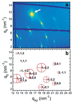
Fig. 4 (a) Grazing incidence X-ray diffraction of a spin-coated 10 g  $l^{-1}$ thin film taken at an incidence angle of 2.0° and (b) calculated diffraction peaks of form 2. The red crosses give the position of the diffraction peaks with the corresponding Laue indices and the area of the red cycles corresponds to the square of the absolute value of the structure factors. The arrow in (a) indicates the (111) diffraction peak of the silicon substrate.
