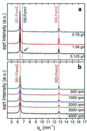
Fig. 2 Specular X-ray diffraction patterns of (a) drop-casted phenoxazine samples with various concentrations without a cover. (b) Spin-coated samples prepared from a 10 g l<sup>-1</sup> solution by applying different spin velocities. Tetrahydrofuran was used as the solvent. Curves are shifted for clarity.
