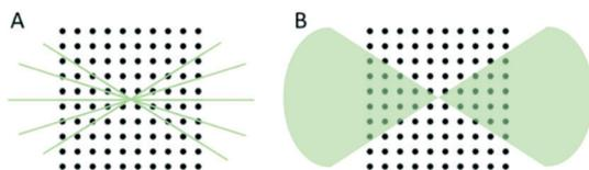
**Fig. 1** Schematic illustration of (A) stepwise and (B) continuous rotation methods for 3D ED data collection. Stepwise methods sample the reciprocal space discretely with point intensities of the reflections are recorded. Continuous rotation methods sample the reciprocal space continuously and take an integral of the intensities over the exposure time.
