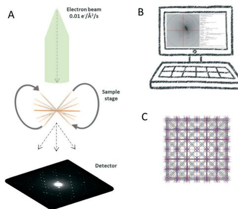
**Fig. 2** Workflow of continuous rotation methods for 3D ED. (A) A fast camera records the diffraction patterns over a desired exposure time while the sample stage is continuously rotated under the electron beam. (B) The raw image data are processed to extract the intensities. (C) Structures of nanometer-sized crystals are solved *ab initio*.
