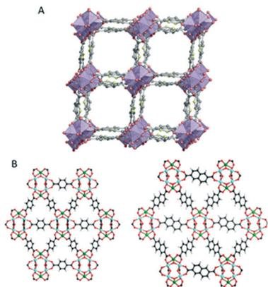
**Fig. 3** (A) The structural model of CAU-23 viewing along the [010] direction. Purple polyhedrons:  $\text{AlO}_6$ ; grey spheres: C; yellow spheres: N. Reproduced from ref. 89 with permission from *Nature Communication*, CC-BY license. (B) The structural models of PCN-415 and PCN-416. Cyan spheres: Zr; green spheres: Ti; red spheres: O; black spheres: C; grey spheres: H. Reproduced from ref. 90 with permission from the American chemical society, copyright 2019.
