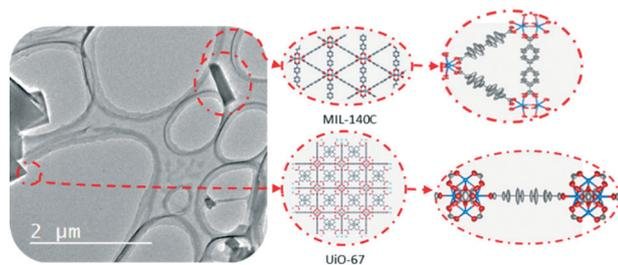
**Fig. 4** The structural models of MIL-140C and UiO-67 which are determined by 3D ED from a mixture. The refinement on ADPs using cRED data reveals small amplitude librations of the linker molecules. Modified from ref. 63 with permission from the American Chemical Society, copyright 2019.
