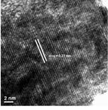
Fig. 11 HRTEM images of the as-prepared SrTiO<sub>3</sub> in [C<sub>3</sub>mimOH][Tf<sub>2</sub>N] with {100} expressed (left) and in [C<sub>4</sub>mim][Tf<sub>2</sub>N] with expression of {110} (right). Reprinted with permission from Wiley-VCH. 156
