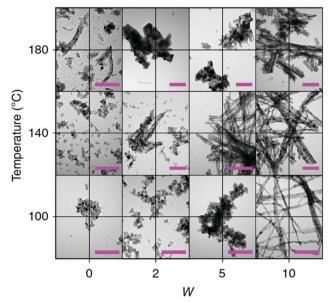
Fig. 18 TEM micrographs as a deep eutectic-solvothermal synthetic phase diagram for CeO<sub>2</sub> nanoparticles post-calcination, where scale bars depict 100 nm, and w is the H2O/[DES] molar hydration ratio. Reprinted with permission from Springer Nature. 307
