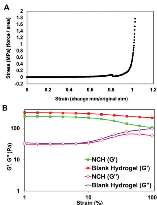
Fig. 7 Mechanical properties of the hydrogels. (A) Compressive stress–strain curves for the NCH system with the load endpoint set at 50 N. (B) Storage ( $G'$ ) and loss ( $G''$ ) moduli obtained using dynamic frequency sweep test from 0.1 to 100  $\text{rad s}^{-1}$ .
