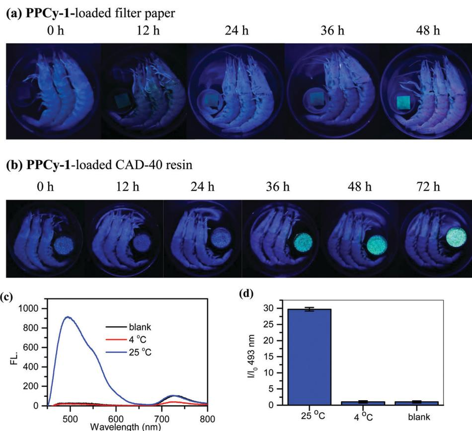
Fig. 8 Monitoring shrimp spoilage at 25 °C by (a) **PPCy-1**-loaded filter paper and (b) **PPCy-1**-loaded CAD-40 resin with fluorescent modes. (c) The emission spectra and (d)  $I/I_0$  at 493 nm of the **PPCy-1**-loaded CAD-40 resin in the absence and presence of shrimp storage at 4 °C and 25 °C for 36 h.
