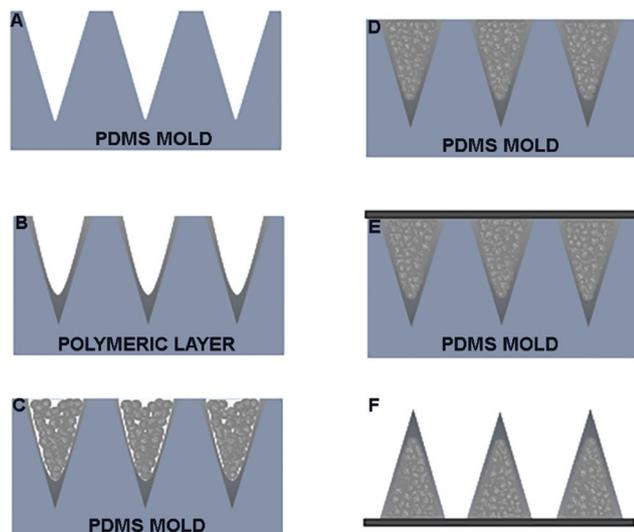
Fig. 5 (A) PDMS mold. (B) Deposition of polymeric solution on PDMS mold. (C) Dried layer. (D) MNs filled with MPs. (E) Compacted and HL applied. (F) MNs extracted from mold. MPs, which are pressed and plasticized by using a non-invasive soft plasticization method previously reported.<sup>19</sup>
