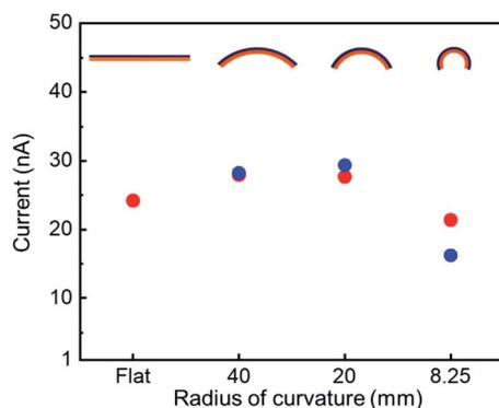
Fig. 5 Current as a function of bending radius of curvature at 10 V (blue circles: bending of a substrate perpendicular to the longitudinal direction ( $a$ -axis) of the underlying  $\text{Cu}(\text{OH})_2$  nanobelts. Red circles: bending of a substrate perpendicular to the short direction ( $c$ -axis) of the underlying  $\text{Cu}(\text{OH})_2$  nanobelts).
