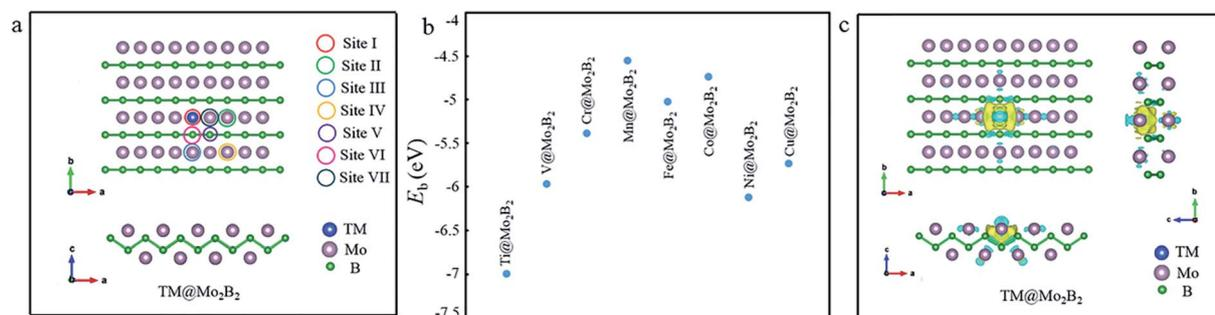
Fig. 1 (a) The structure and seven possible active sites of  $\text{TM@Mo}_2\text{B}_2$ . (b) The binding energy diagram of different  $\text{TM@Mo}_2\text{B}_2$  (TM = Ti, V, Cr, Mn, Fe, Co, Ni and Cu). (c) The charge density difference of  $\text{TM@Mo}_2\text{B}_2$ , where yellow and blue regions indicate the charge density accumulation and depletion, respectively.
