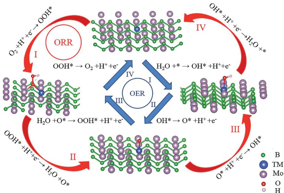
Fig. 3 Elementary reaction steps of the OER and ORR process for TM@Mo<sub>2</sub>B<sub>2</sub> at site I.
