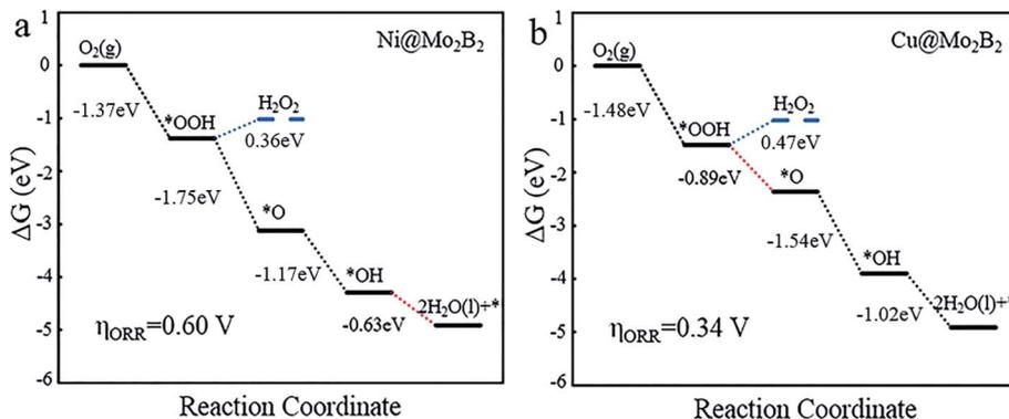
Fig. 5 The Gibbs free energy diagrams for the  $4e^-$  and  $2e^-$  ORR processes of (a) Ni@Mo<sub>2</sub>B<sub>2</sub> and (b) Cu@Mo<sub>2</sub>B<sub>2</sub> at site I, where the blue lines represent the  $2e^-$  ORR process, the black lines represent the  $4e^-$  ORR process, and the red dashed lines represent the most energy-consuming step of the ORR.
