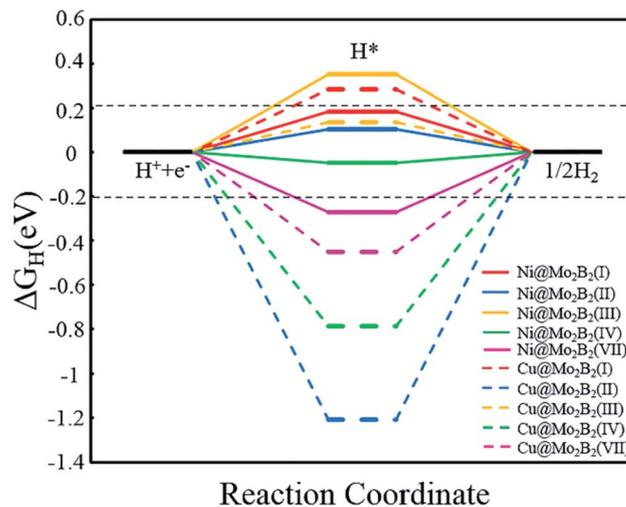
Fig. 7 Calculated Gibbs free energy diagram for the HER at different sites for Ni@Mo<sub>2</sub>B<sub>2</sub> and Cu@Mo<sub>2</sub>B<sub>2</sub> for a hydrogen coverage of 1/16. The two horizontal black dashed lines correspond to  $|\Delta G_{\text{H}}| = 0.2$  eV.
