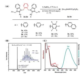
Fig. 2 (A) Preparation of  $[Au_{13}(bisNHC)_5X_2]X_3$  nanoclusters  $[3a-e]X_3$ (B) ESI-MS of [3a]Cl<sub>3</sub>; (C) UV-vis absorbance (red), photoluminescence excitation (black) and emission (green) spectra of [3a]Cl3 in dichloromethane.
