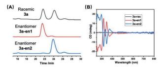
Fig. 5 Enantioseparation and characterization of chiral Au<sub>13</sub> nanoclusters: (A) chromatogram showing the enantioseparation of *rac-3a* by chiral HPLC using UV-vis detection at 350 nm; (B) CD spectra of the two chiral enantiomers separated by HPLC and *rac-3a* for comparison.
