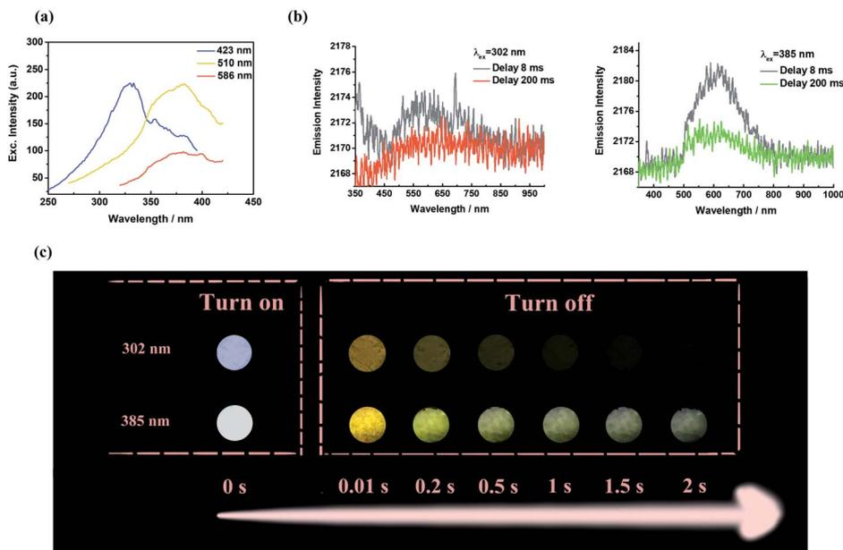
Fig. 5 (a) The excitation spectra of 3-SPhF at different excitation wavelengths; (b) phosphorescence spectra and (c) photographs of 3-SPhF under 302 nm and 385 nm excitations.
