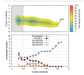
Fig. 5 (Upper panel) Free energy surface for the binding of Pb reconstructed from one out of two *ab initio* metadynamics simulations (see Fig. S7† for both) started from the end (unbound state, S > 1.8) of the simulation in Fig. 4. In the shaded area -S < 1.2 – the bias is not representative of the free-energy. (Lower panel) Evolution of the coordination of Pb with oxygen atoms belonging to water and to different organic functional groups as function of the S path coordinate.
