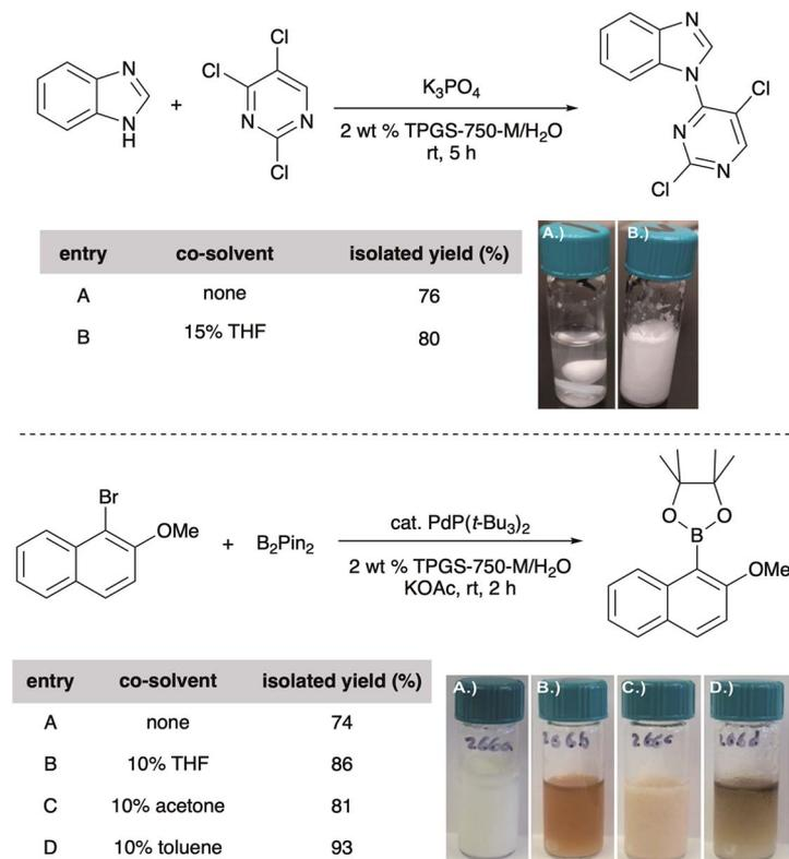
Fig. 12 Effect of co-solvents on yields and processability.
