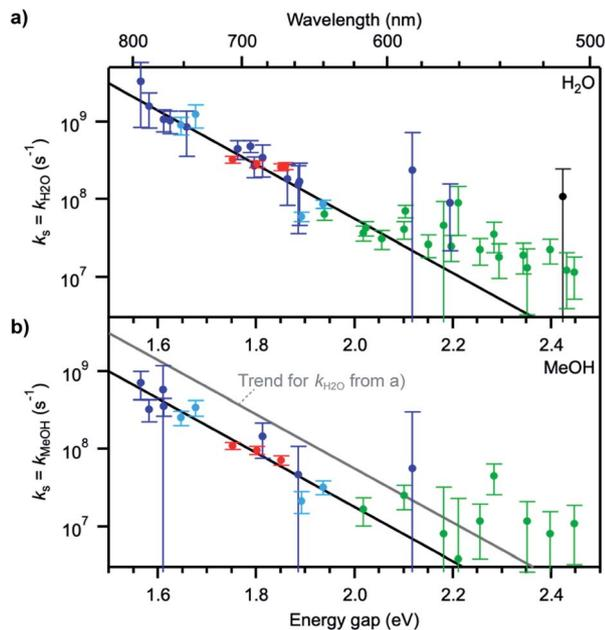
Fig. 4 (a) Solvent quenching rate constant in water and (b) in methanol as a function of the  $S_0$ – $S_1$  energy gap of each fluorophore. The colour coding of the data points is the same in (a) and (b). Black lines represent trends to the data points at energy gaps up to  $\sim 2.1$  eV. The grey line in (b) indicates the trend for  $k_{H_2O}$  determined in (a). Error bars were determined from the estimated measurement uncertainty on the fluorescence lifetime.
