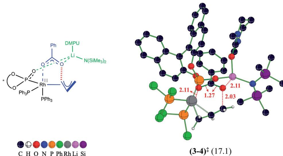
Fig. 1 Optimized geometry of the transition state  $(3-4)^\ddagger$  for the C–O bond oxidative addition, leading to the formation of a Rh- $\pi$ -allyl intermediate. Relative Gibbs free energy (in kcal mol<sup>-1</sup>) given in parentheses is with respect to the separated reactants with **B1** as the active catalyst. Distances are in Å.
