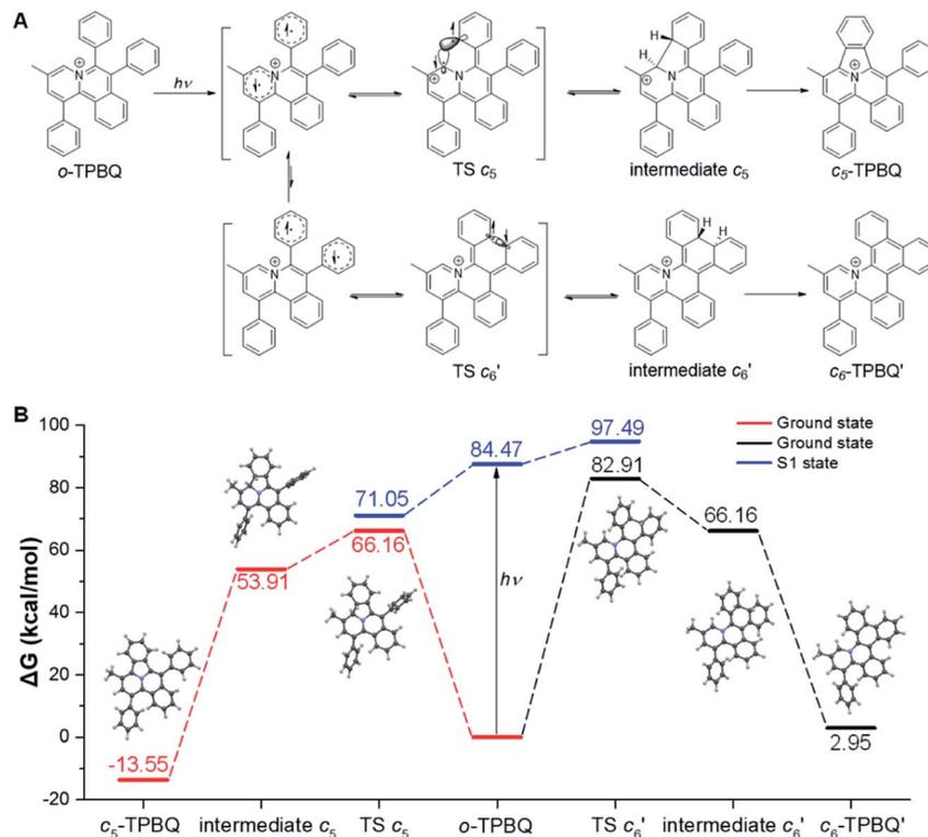
Fig. 3 Proposed photoreaction mechanism of *o*-TPBQ. (A) Possible reaction pathway. (B) Gibbs free energy of the ground and S1 state of the five-membered ring product ( $c_5$ -TPBQ) and six-membered ring product ( $c_6$ -TPBQ') formation process. The counteranions are omitted for clarity.
