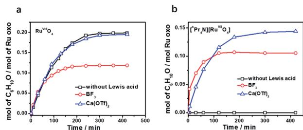
Fig. 1 Time traces for cyclohexane oxidation by (a)  $\text{RuO}_4/\text{Lewis acid}$  and (b)  $\text{RuO}_4^-/\text{Lewis acid}$  in  $\text{CH}_3\text{CN}$ . Conditions:  $\text{RuO}_4$  or  $[^n\text{Pr}_4\text{N}][\text{RuO}_4^-]$  (0.01 M), Lewis acid (0.04 M), cyclohexane (1.0 M) at 23 °C.
