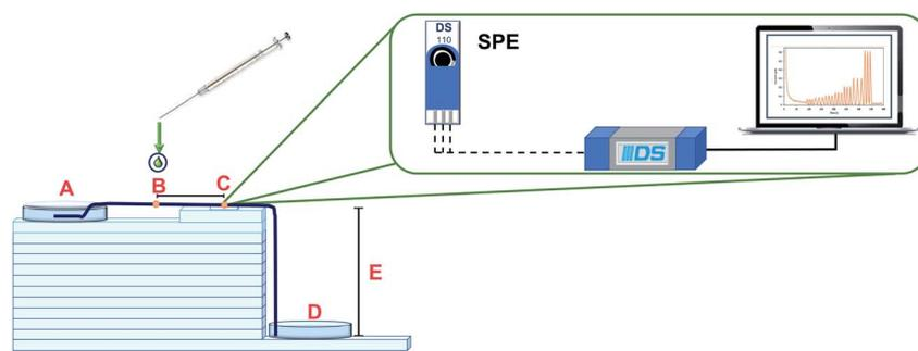
**Fig. 7**  $\mu$ FIA device configuration for LMG determination using amperometric detection (0.8 V), where A = electrolyte inlet, B = injection point, C = detection zone, D = electrolyte outlet and E = height of the device. The detector used consists of a carbon screen printed electrode (SPE) and the flow is directed through the system using the henequen fiber as a microchannel.
