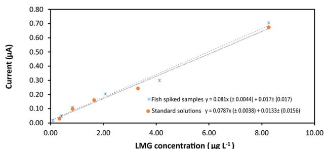
Fig. 6 Calibration plot of LMG. Comparison of the analytical sensitivity (slope) using standard solutions and fish spiked samples. Linear interval 0.082–8.262  $\mu\text{g kg}^{-1}$ .
