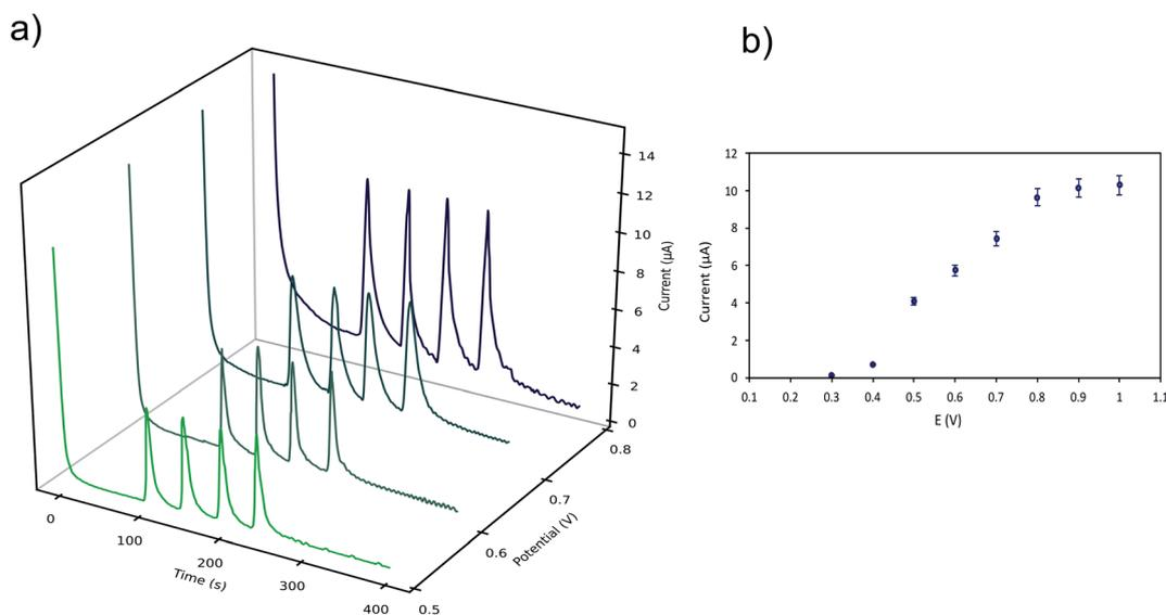
Fig. 4 Effect of the oxidation potential applied on the analytical response *vs.* Ag reference electrode (LMG concentration used was 1.0 mM in 50 mM ammonium acetate buffer pH = 4.0 ± 0.02 with ACN (40% v/v) and Tween-80 (1% v/v)). (a) Amperometric determination of LMG on the  $\mu$ FIA system using different oxidation potentials (0.5–0.8 V). (b) Hydrodynamic voltammetry *I-E* curve obtained for a 3  $\mu$ L injection of LMG solution.
