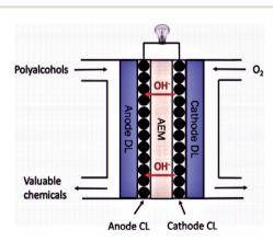
Fig. 4 Schematic diagram of the Anion Exchange Membrane Fuel Cell. Reproduced from ref. 44, Copyright 2017, Elsevier [CL = catalyst layer, DL = diffusion layer, AEM = anion exchange membrane].
