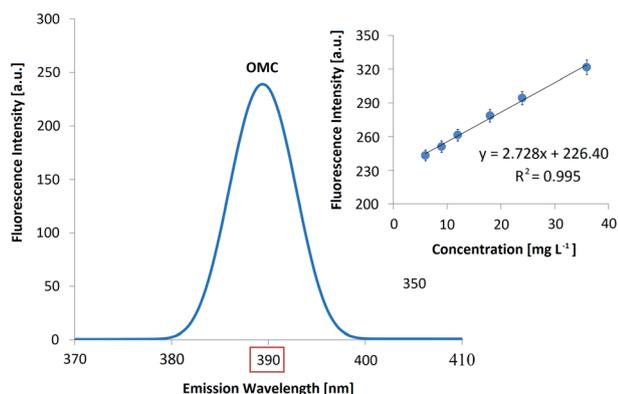
Fig. 3 Fluorescence spectrum corresponding to a standard solution of OMC (30 mg L<sup>-1</sup>). The characteristic maximum of signal at 390 nm and the calibration curve in the concentration range of 6.0–36.0 mg L<sup>-1</sup> are shown. It is important to note that OA is not fluorescent around 390 nm.
