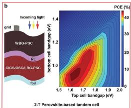
Fig. 3 Structure and simulated efficiency of flexible tandem solar cells. (a) 4-T tandems and (b) 2-T tandems. Reproduced with permission.<sup>43</sup> Copyright 2020, Wiley-VCH.
