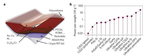
Fig. 4 Power-per-weight analysis. (a) Schematic diagram of the ultrathin perovskite solar cell. (b) Power-per-weight of various photovoltaic technologies. Reproduced with permission. Copyright 2015, Springer Nature.
