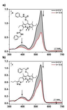
**Fig. 2** Evolution of UV-vis spectra during the photoreaction of BODIPY-model compounds **5** (a) and **6** (b) in aerated methanol solutions  $(5.3 \times 10^{-5} \text{ M} \text{ and } 4 \times 10^{-5} \text{ M}, \text{ respectively})$  upon 505 nm LED irradiation for the indicated time.
