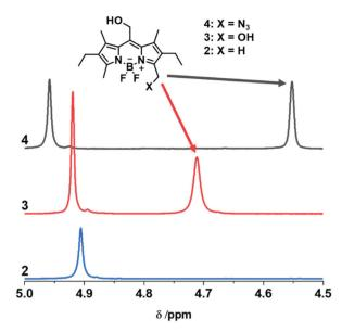
Fig. 3  $\,^{1}$ H-NMR spectra in CDCl $_{3}$  of the hydrolysed BODIPY compound 2 (blue), the BODIPY-diol compound 3 (red) and the BODIPY-azide compound 4 (black) showing the proton signals arising upon the substitution at position 3 at 4.71 ppm and 4.55 ppm for the diol and the azide, respectively.
