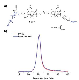
Fig. 6 Loading of the BODIPY 4 or 7 onto the poly(organo)phosphazene. (a) Scheme of the reaction of BODIPY 4 or 7 with poly(organo) phosphazene. (b) SEC-traces of the UV-vis (540 nm) and the refractive index detectors, showing an overlap of the signals and indicating a successful loading of the BODIPY compound 7 onto the poly(organo)phosphazene carrier. (i)  $CuSO_4 \cdot 5H_2O$ , (+)-L-Na ascorbate, DCM/H<sub>2</sub>O.
