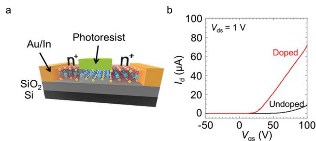
**Fig. 4** (a) Schematic diagram of an n<sup>+</sup>/i/n<sup>+</sup> patterned device with a photoresist coating. (b) Transfer curves of the device with the photoresist coating before and after the doping using 100 mM dopant solution.
