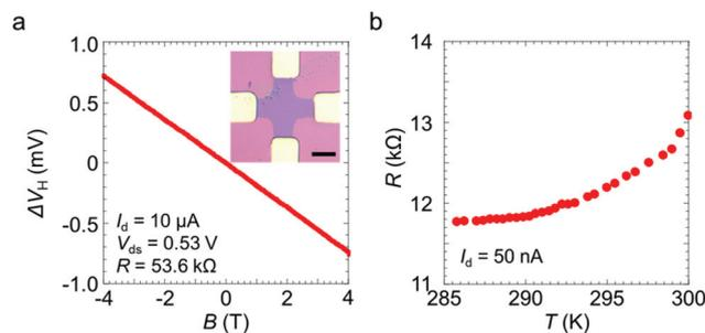
Fig. 2 (a) Magnetic field dependence of the Hall voltage for the doped monolayer  $\text{MoS}_2$  using  $100 \text{ mM}$  dopant solution at room temperature. The inset is an optical image of the sample. The scale bar is  $10 \mu\text{m}$ . (b) Temperature dependence of the electrical resistance for the doped monolayer  $\text{MoS}_2$  using  $100 \text{ mM}$  dopant solution.
