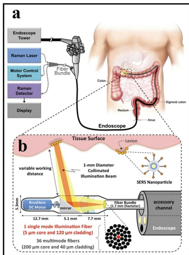
**Fig. 20** Schematic representation of a Raman-imaging system in combination with white-light endoscopy. (a) The design and construction of the device allows it to pass through the accessory channel of a clinical endoscope. (b) An expanded view of the distal end of the device. Reproduced with permission.<sup>262</sup> Copyright 2015, Garai *et al.*
