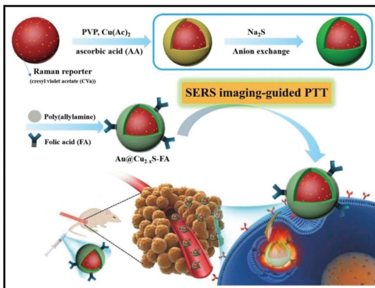
**Fig. 19** Schematic of the development of Au@Cu<sub>2-x</sub>S-FA core-shell NPs and their *in vitro* and *in vivo* SERS application for identification and photothermal therapy of cancer cells at the cellular level. Reproduced with permission.<sup>261</sup> Copyright 2018 WILEY-VCH Verlag GmbH & Co. KGaA, Weinheim.
