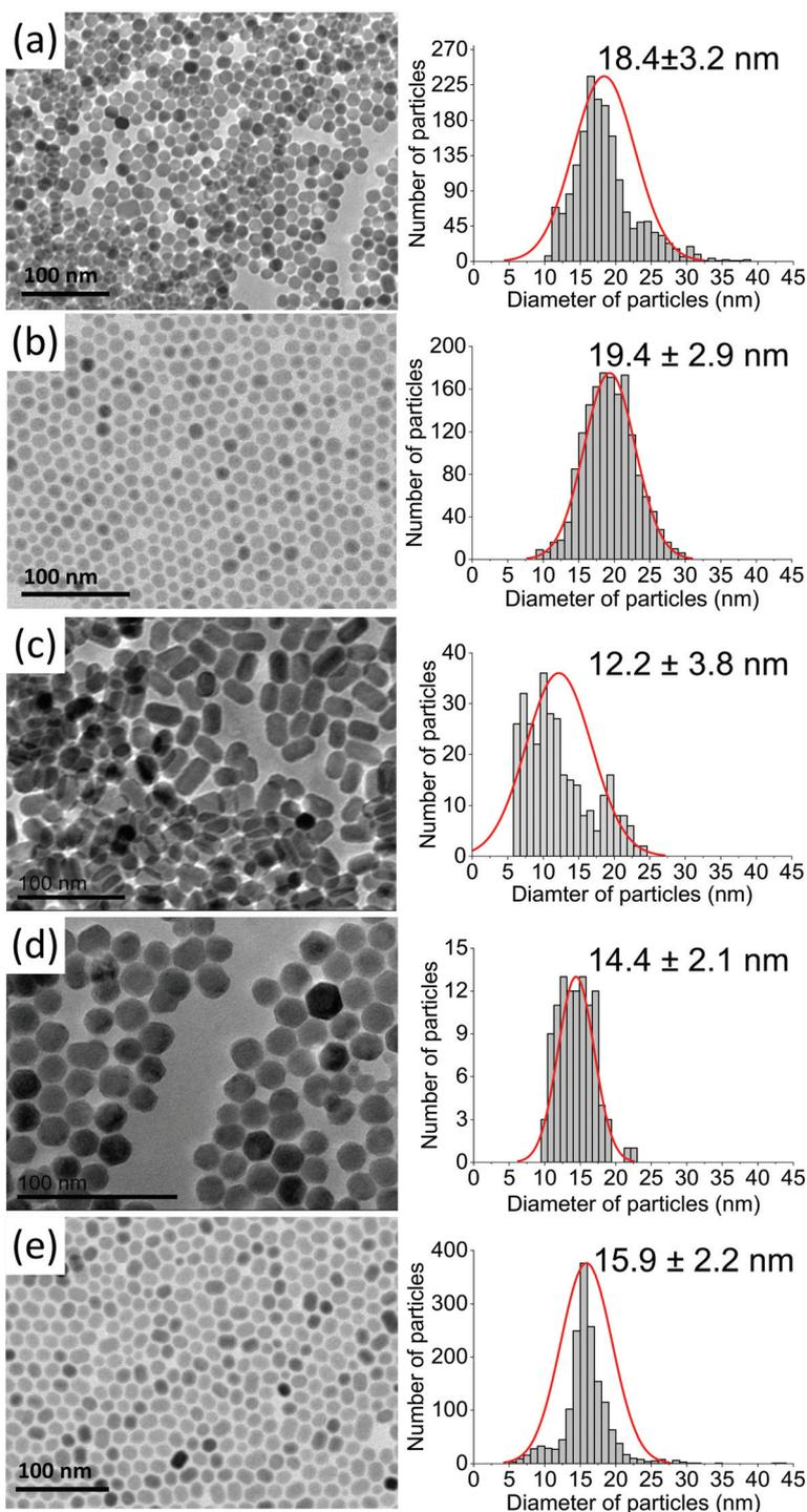
Fig. 2 TEM images recorded for (a)  $\text{NaYF}_4:2\%\text{Tm}^{3+}@NaYF_4$ , (b)  $\text{NaYF}_4:2\%\text{Tm}^{3+},5\%\text{Er}^{3+}@NaYF_4$ , (c)  $\text{NaYF}_4:2\%\text{Tm}^{3+}@NaYF_4:5\%\text{Er}^{3+}$ , (d)  $\text{NaYF}_4:18\%\text{Yb}^{3+},2\%\text{Tm}^{3+}@NaYF_4$ , and (e)  $\text{NaYF}_4:18\%\text{Yb}^{3+},2\%\text{Tm}^{3+}@NaYF_4:5\%\text{Er}^{3+}$  NPs.
