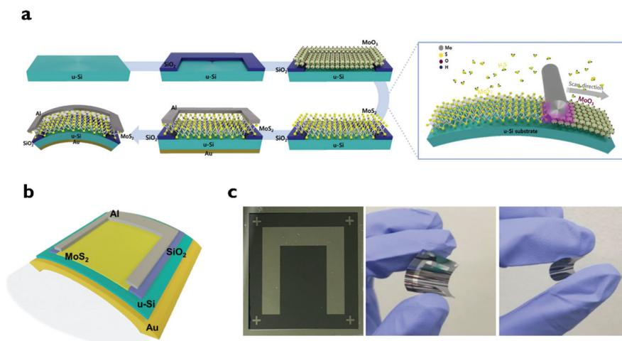
**Fig. 1** (a) Schematic fabrication process of the MoS<sub>2</sub>/Si heterojunction-based photodetector. (b) Illustration of flexible MoS<sub>2</sub>/Si photodetector. (c) Optical image of the real device and under bending conditions.
