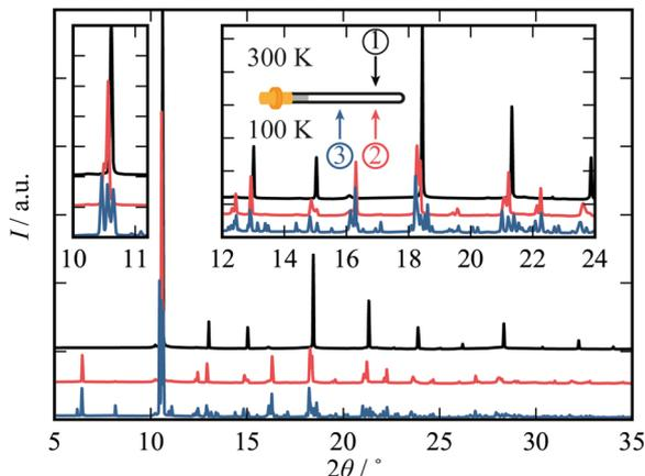
Fig. 3 Diffraction patterns ( $\lambda = 0.82484 \text{ \AA}$ ) collected for a sample of  $\text{Cd}(\text{CN})_2$  at 300 K (black) and in the same position at 100 K (red) and at 100 K having been translated (blue = minimal prior exposure). The nature of the phase transition is clearly affected by irradiation prior to cooling.
