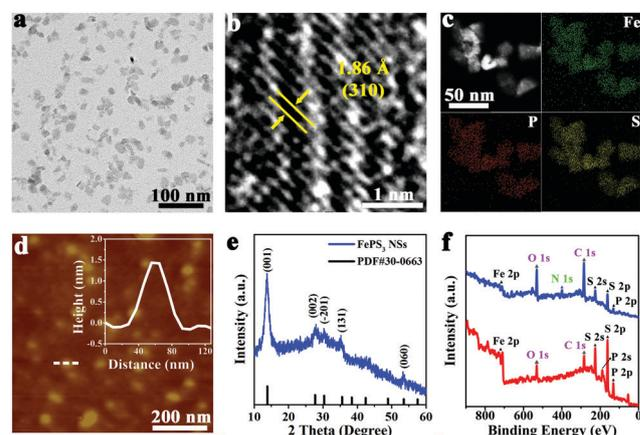
**Fig. 1** (a) TEM image, (b) HRTEM image, (c) HAADF-STEM image and the corresponding EDS elemental mapping images, (d) AFM image with height profile, and (e) XRD pattern of  $\text{FePS}_3$  NSs. (f) XPS survey spectra of  $\text{FePS}_3$  NSs (blue) and bulk  $\text{FePS}_3$  (red).
